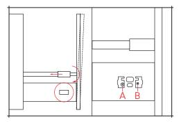
When installing with a countertop, offer the countertop to the wall mounted units and mark the position of the waste and tap holes. Place the countertop on top of a surface such as MDF and make the required holes. All holes made into wood should be sealed with a PVA or Oil Based Paint to seal the wood.
