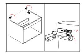
5. Secure the unit to the mounting plates using the hooks fitted on the unit. The unit can then be adjusted. Screw A adjusts the height. Screw B adjusts the depth.
